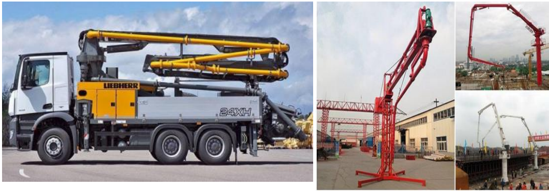
Gambar 1. Truck Mounted Concrete Pump dan Portable mast and boom.[9].
