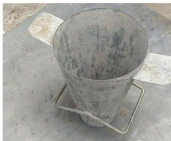
Gambar 1. Kerucut Abrams
