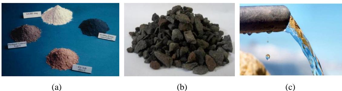
**Gambar 2** Material penyusun beton porous, a) *cementitious materials*, b) agregat kasar, c) air
